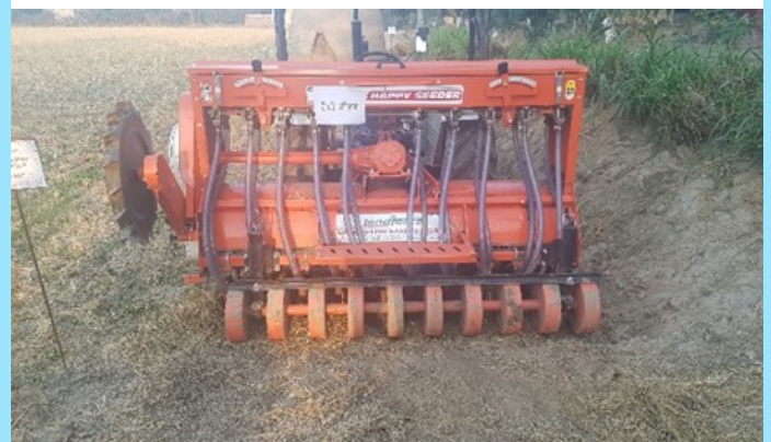
The Happy Seeder allows farmer to direct drill the wheat into the smashed rice stubble
